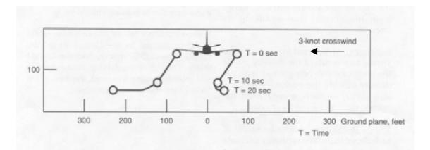
FIGURE 7. EFFECT OF 3-KNOT CROSSWIND ON VORTICES FROM LOW FLYING AIRCRAFT
