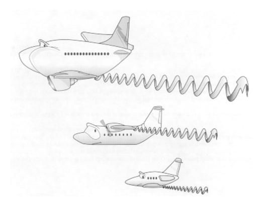
FIGURE 3. WAKE VS. AIRCRAFT WEIGHT
