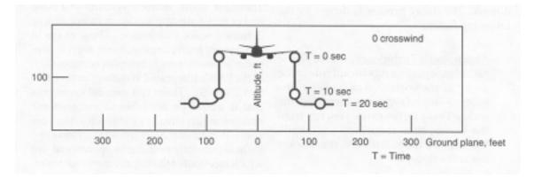
FIGURE 6. MOVEMENT OF VORTICES FROM LOW FLYING LARGE AIRCRAFT
