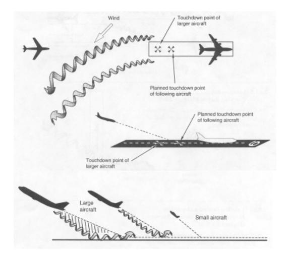
FIGURE 4. ROTATION AND TOUCHDOWN POINTS OF PRECEDING AIRCRAFT
