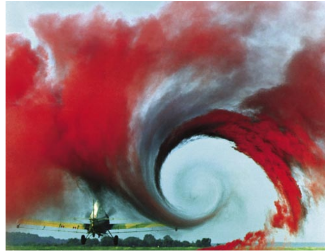
Figure 4-7. Wingtip vortex from a crop duster.
