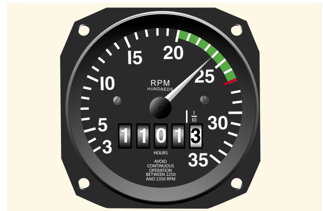
Figure 6-8. Engine rpm is indicated on the tachometer.
