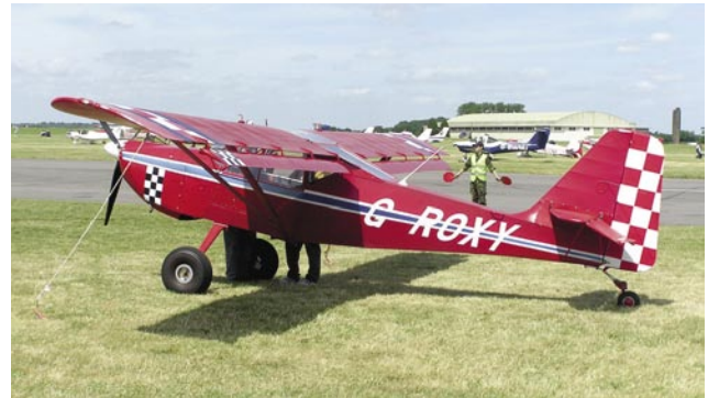
Figure 5-9. Flaperons on a Skystar Kitfox MK 7.
