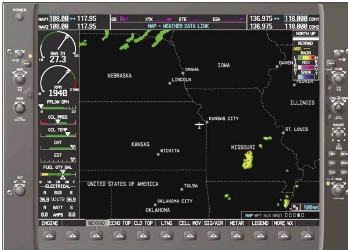
Figure 12-24. NEXRAD radar display (500 mile range). The individual color gradients can be easily discerned and interpreted via the legend in the upper right corner of the screen. Additional information can be gained by pressing the LEGEND soft key, which displays the legend page.
